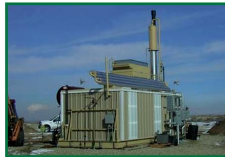
*Quantum Leap Natural Gas Dehydration Technology (QLT) at a Colorado gas processing facility*
