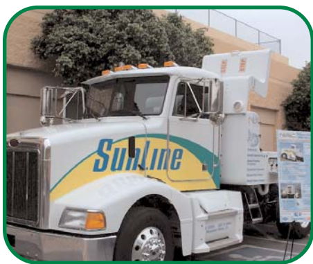
Fuel cell-powered heavy duty truck.
