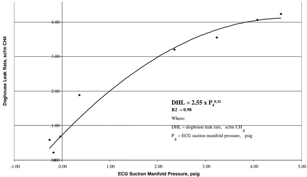
**Figure 4. Leak rate versus ECG suction pressure.**
