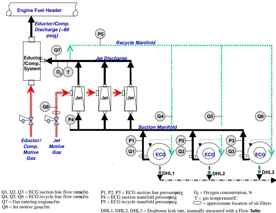
Figure 3. The as-built SAS and measurement system at test site.
