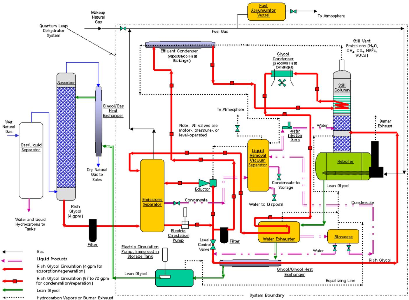
Figure 1. Schematic of QLD Natural Gas Dehydration Technology
