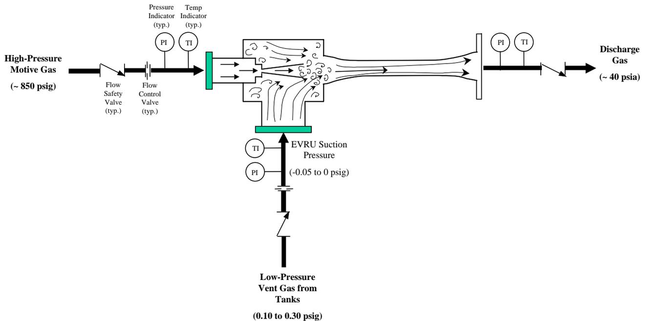
Figure 1. Schematic of the COMM EVRU
